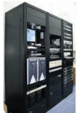
Two hard disk servers are mounted on an equipment rack.
