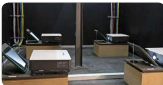
4x PT-D5500 projectors used for the on-floor backprojection
